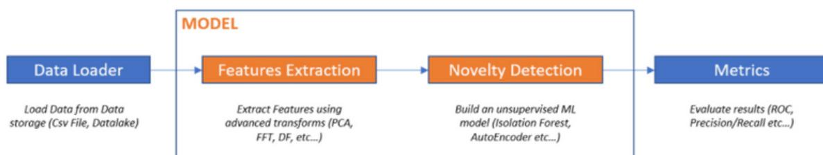
Figure 1 : Diagram of a predictive model
